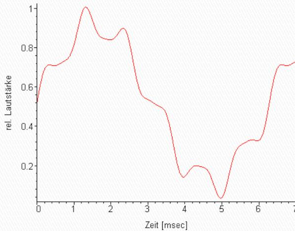
Nutzsignal: Sinuskurven 160 Hz + 960 Hz + 1750 Hz
